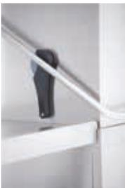
**PROGLIDE:** The hood slides smoothly on anti-friction guides and is activated by a system of levers, without buckling or jamming if the handle is grasped from a corner. The weight of the hood is counter-balanced and lifting force is a mere 3 kg, thus reducing operator fatigue and increasing productivity. The hood is of the double skin insulated type to reduce heat and noise emissions.
