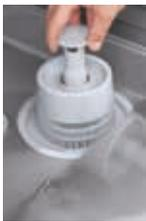
**ARCHIMEDES:** During rinsing, clean water is pumped into the tank to replace the dirty water. With a conventional gravity waste, the clean water floats on top of the heavier dirty water so that pumping in three litres one goes directly to the drain. ArchiMedes, exploits the principle of communicating vessels, reducing losses by 38% to 17%.
