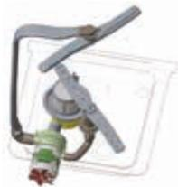
**DUO FLO:** A conventional pump has an inlet (from the tank) and an outlet towards the two spray arms: the flow of water must be distributed using a T or Y connector. Our research has revealed that this is where 25-30% of power is lost. We have eliminated the problem with a simple solution: the pump has one inlet but two outlets without any T divider. Loss is not only reduced but completely eliminated, with also a 50% reduction in noise.
