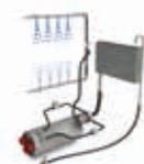
**PRORINSE CONSTANT RINSING:** It uses a 200 W rinsing pump to guarantee the pressure and flow rate of rinsing whatever the supply conditions of the water network. Feeding at the boiler takes place through a "break tank" anti-pollution device, which is type-approved in compliance with the English WRAS regulation.
